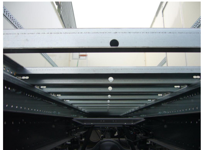
Cross-members pre-drilled for a wire shield tube
