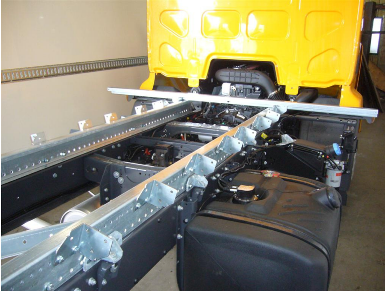
Bonding between cross-members and main beams with pre-drilled angle bars
